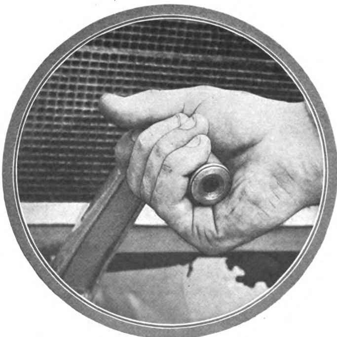
Fig. 2.—Operator in the act of starting the motor, showing how the starting handle is too short and how the roller slides over the rivet
